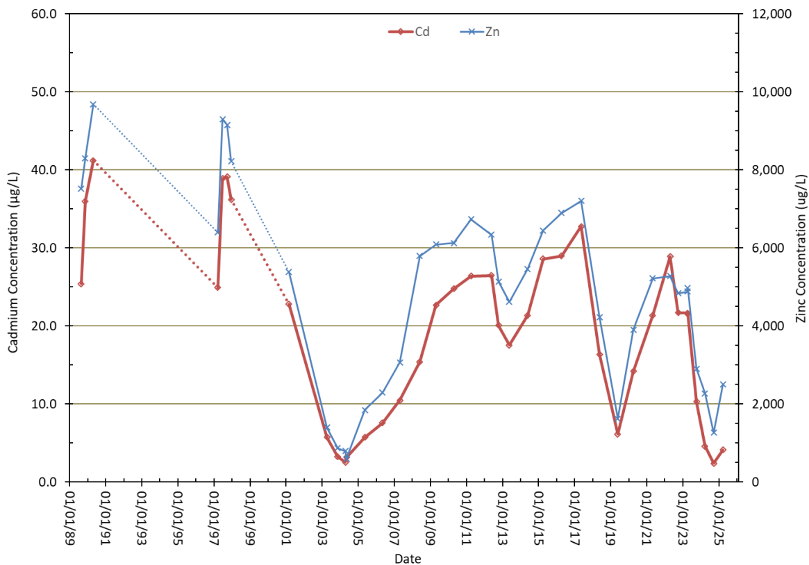
Figure 2-25. Cadmium and zinc concentration trends in well GS-44S. The DEQ-7 human health water-quality standard for cadmium in groundwater is 5 µg/L, and for zinc is 2000 µg/L.
