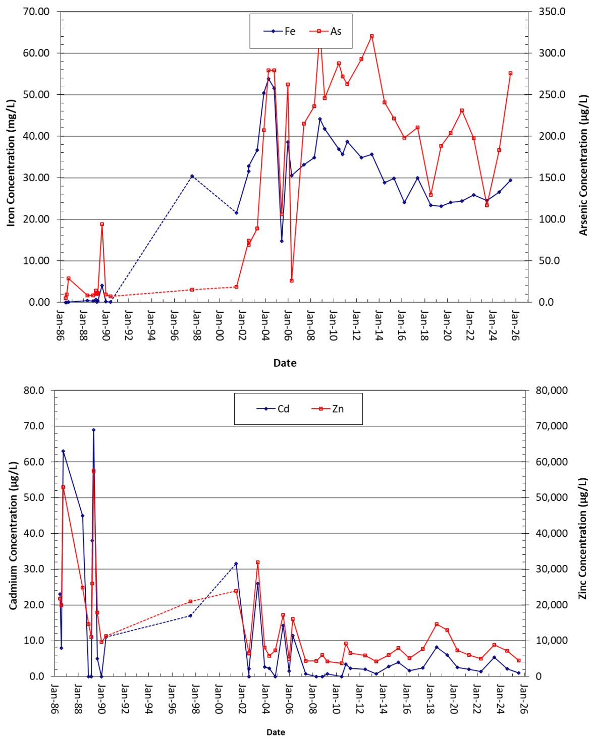
Figure 3-7. Anselmo Mine iron and arsenic concentrations (top) and cadmium and zinc concentrations (bottom) over time.
